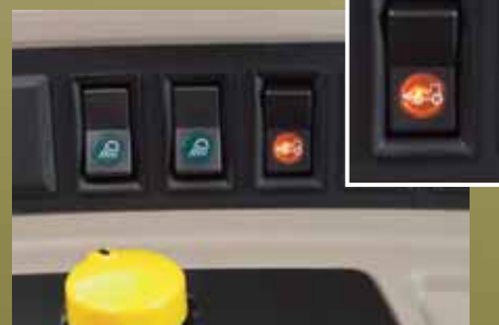
(Picture shows an Electro-Hydraulic on the go switch on F12/R12 models)
